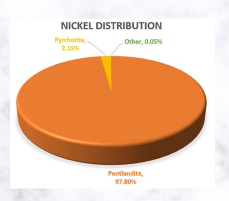
Pentlandite was the main nickel mineral observed. Nickel in the form of pentlandite can generally be recovered with gravity and/or flotation methods.
